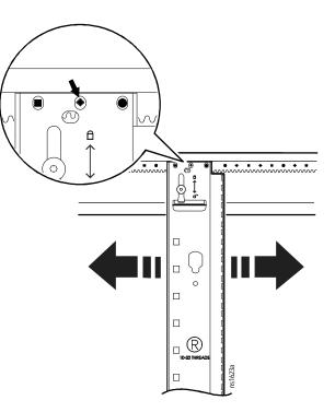
4. Lock top and bottom of the vertical mounting rail.
